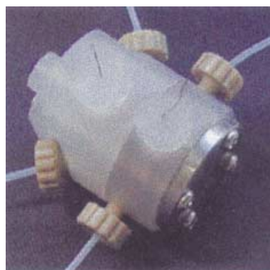
Figure 4. An electrochemical microflow reactor for the “cation flow” method.
